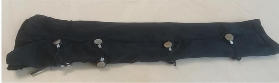
**FIGURE 3.** Physical prototype of the lymphometer.
